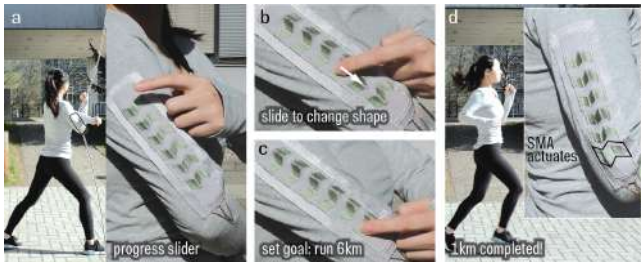
Figure 19: (a) The shape-changing progress slider allows users to (b-c) easily set a running goal. It (d) actuates to change shape for each km the user runs to give visuo-haptic feedback of the running progress.
