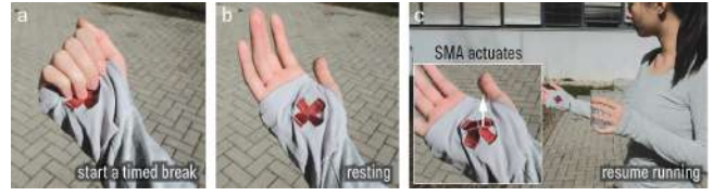
Figure 20: The user starts a timed break by (a) a simple clench and gets notified through the SMA-actuated shape change when the break has ended.
