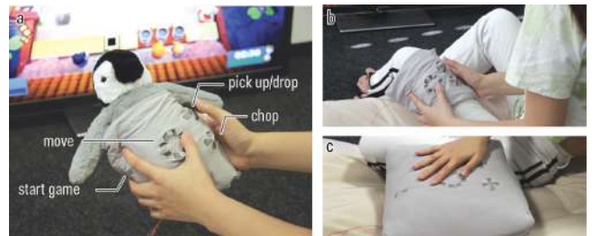
Figure 21: We used Embrogami structures to design a (a) textile-based game controller that can (b) be wrapped around anywhere to allow playing in changing physical contexts or (c) be flattened to disable the controls and blend in with other furniture.
