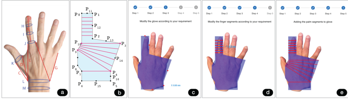
Fig. 7. MediKnit design tool provides: (a) Visual guidance for thirteen hand measurements for customization; (b) Backend algorithm converts the measurements to 18 coordinate points; (c) and (d) A glove template is generated based on these coordinates, with options for therapists to adjust both the template and SMA channels; (e) The design tool then creates a machine-readable file.
